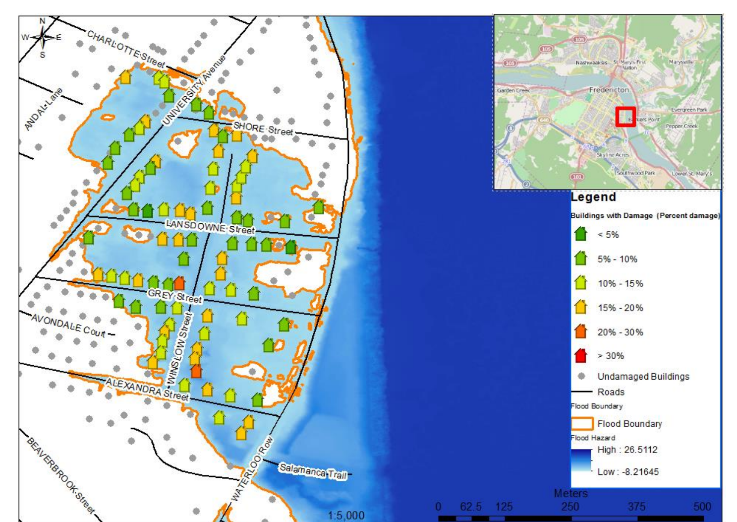
Partial results from Hazus loss estimation using data derived via ETL models and python scripts
